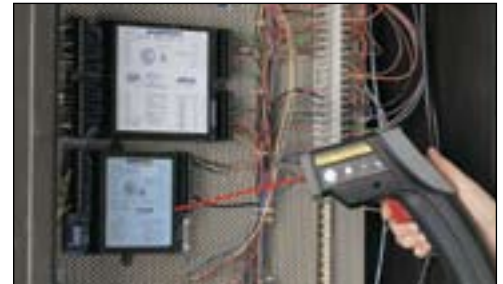
Measuring panels that are difficult to evaluate with contact sensors.
