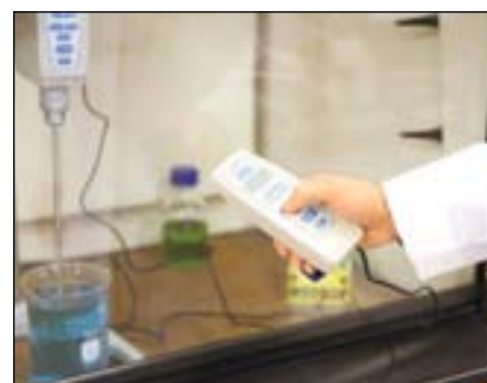
Safely adjust mixer setting without opening the fume hood.
